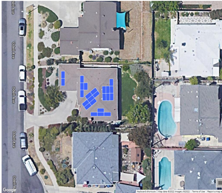
PANEL TYPE 24x LA Solar (450 Watts)
